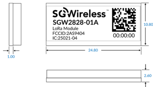
Figure 3. SGW2828 Mechanical Information
