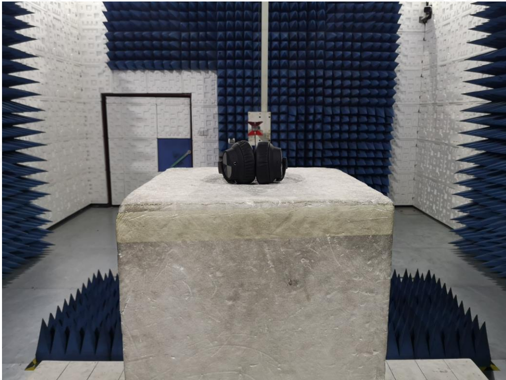
RADIATED EMISSION TEST SETUP ABOVE 1GHZ
