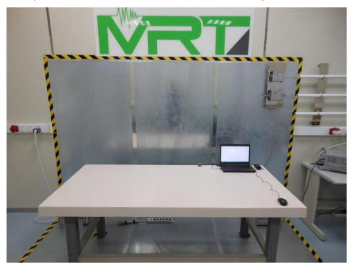
Test Mode 1 Description: Back View of Conducted Emission Test Setup
