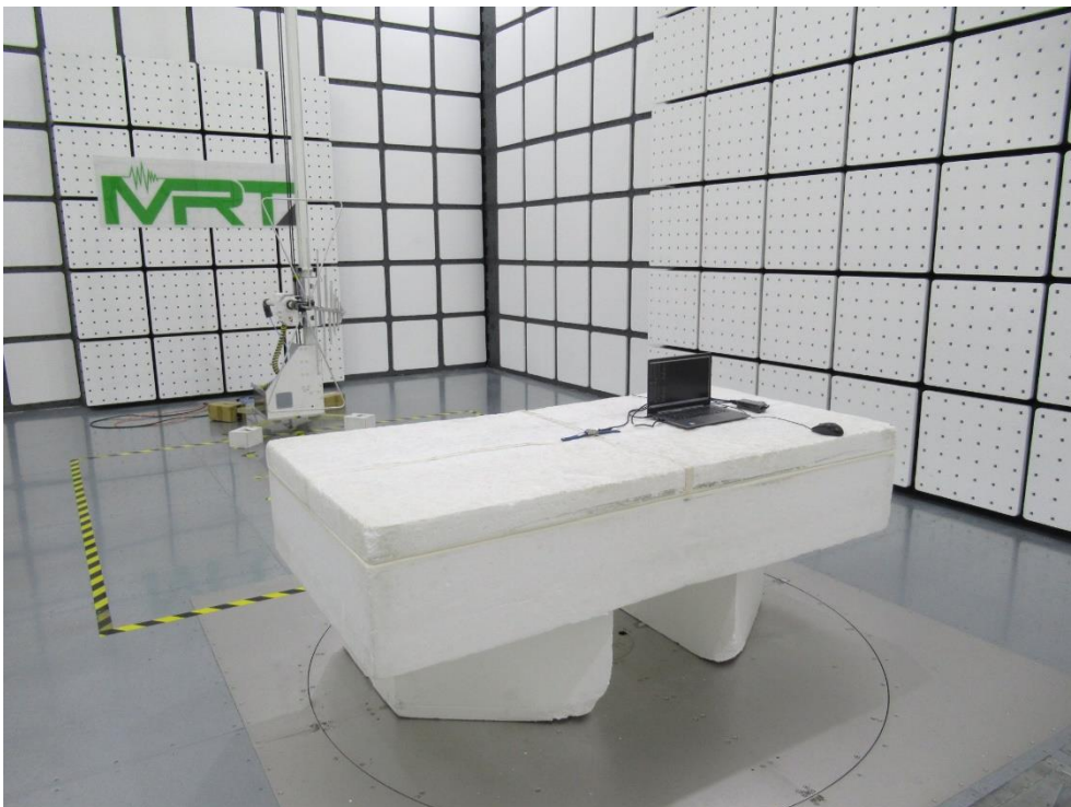
Description: Radiated Emission Test Setup for 30MHz~1GHz (S2.3 Steel)
