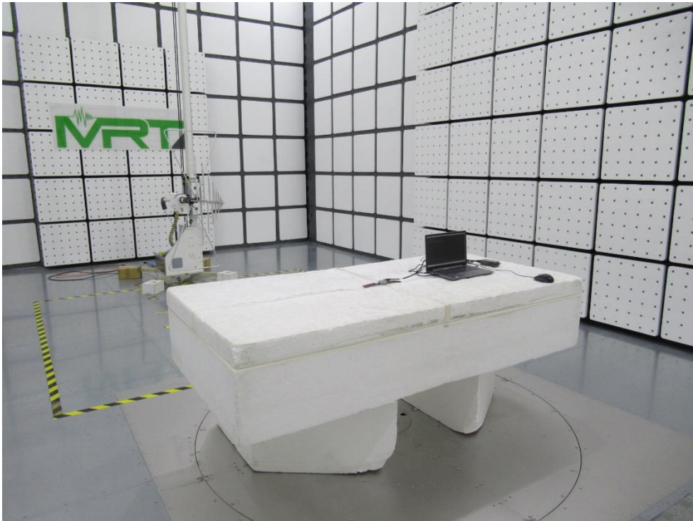
Description: Radiated Emission Test Setup for 30MHz~1GHz (S2.3 Steel)
