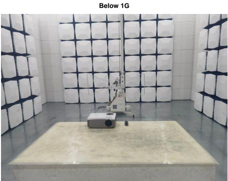
Radiated Emissions Test Setup
