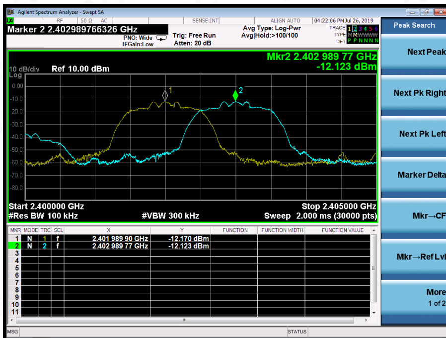
TEST PLOT FOR FREQUENCY SEPARATION
