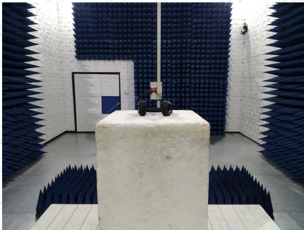
RADIATED EMISSION TEST SETUP ABOVE 1GHZ
