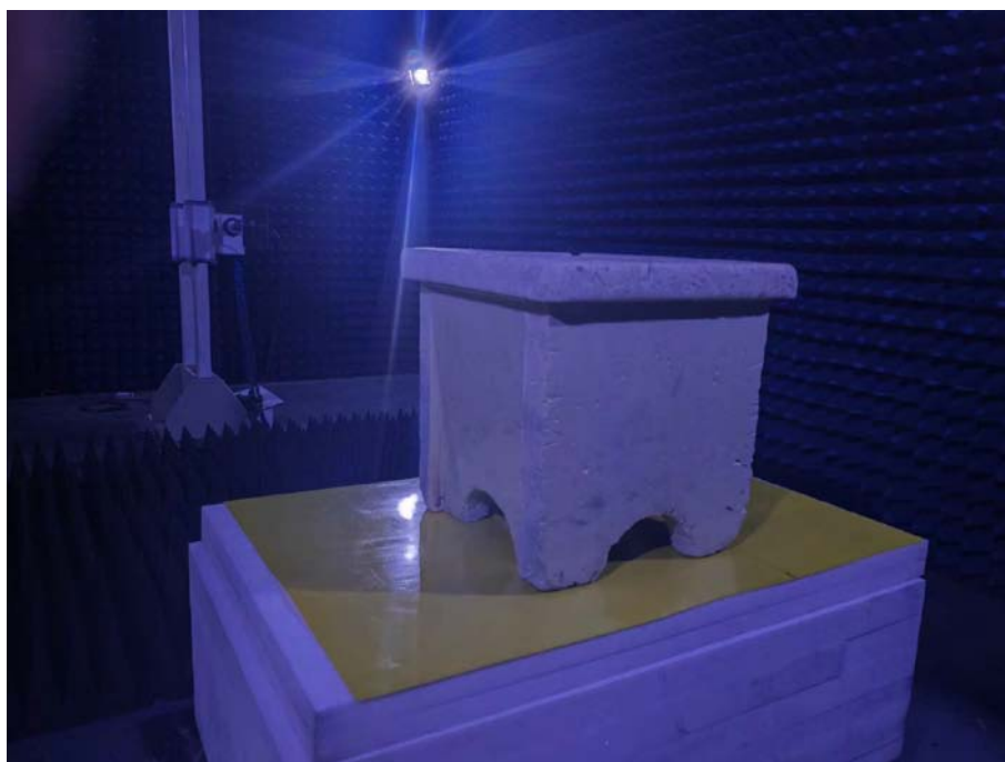
Photo of Radiated Emission Measurement Above 1GHz
