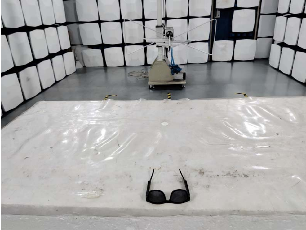
Radiated emission test view
