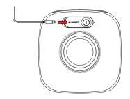
Insert the other end of the USB cable into a suitable USB charging adapter.
