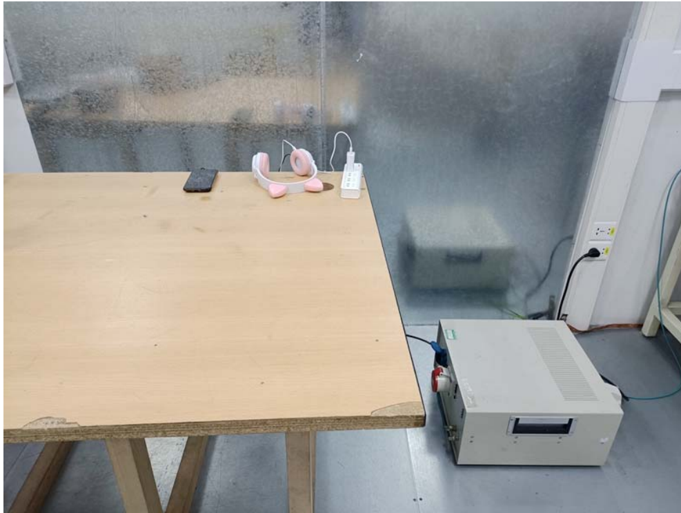
Conducted Emission Test Setup:
