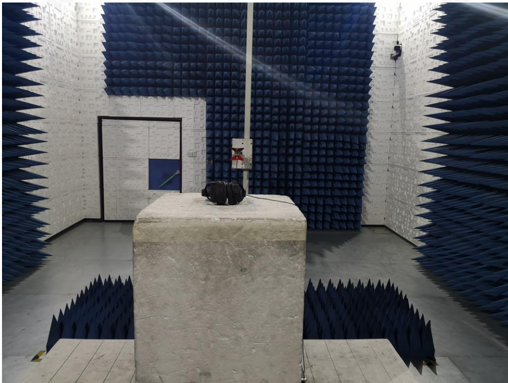
RADIATED EMISSION TEST SETUP ABOVE 1GHZ
