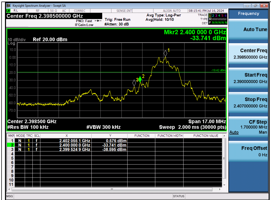
Test_Graph_LE2M_ANT1_2402_2Mbps_Lower Band Edge Emissions
