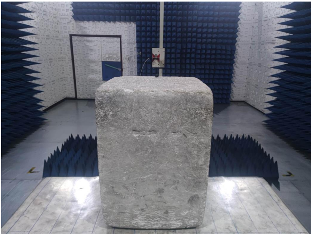
RADIATED EMISSION TEST SETUP ABOVE 1GHz
