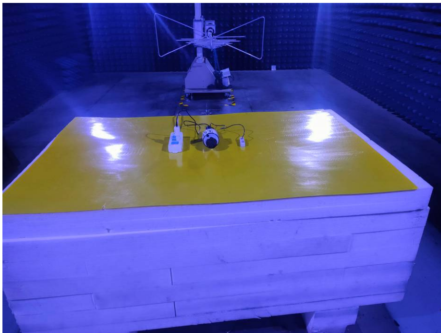
Photo of Radiated Emission Measurement (Above 1G)
