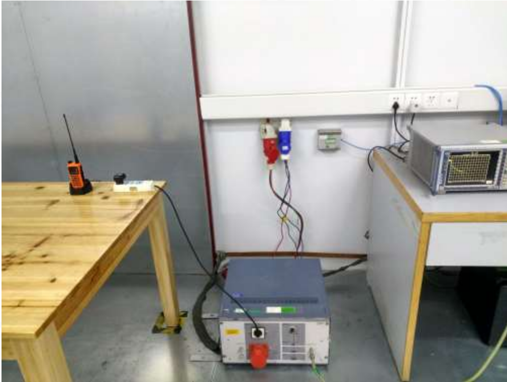
RADIATED EMISSION TEST SETUP-BELOW 1GHZ
