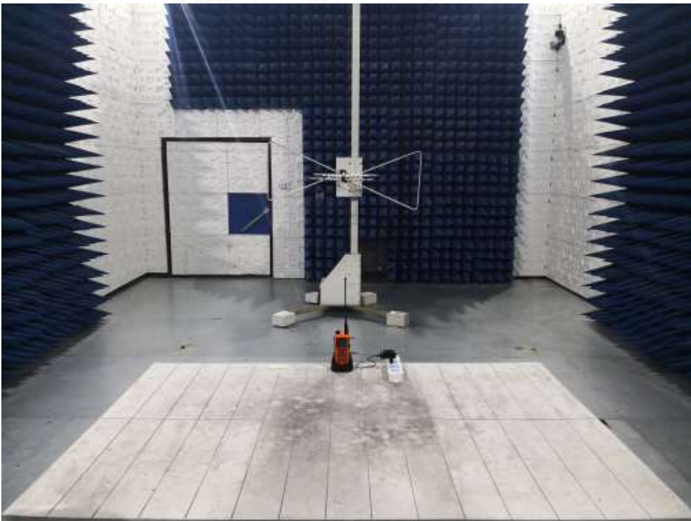
RADIATED EMISSION TEST SETUP-BELOW 1GHZ
