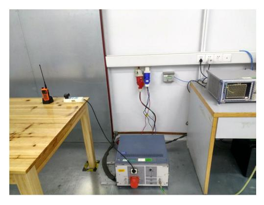
RADIATED EMISSION TEST SETUP-BELOW 1GHZ
