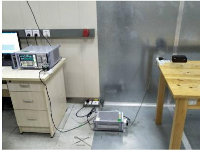
Radiated Spurious Emissions Test Frequency From 30MHz-1000MHz
