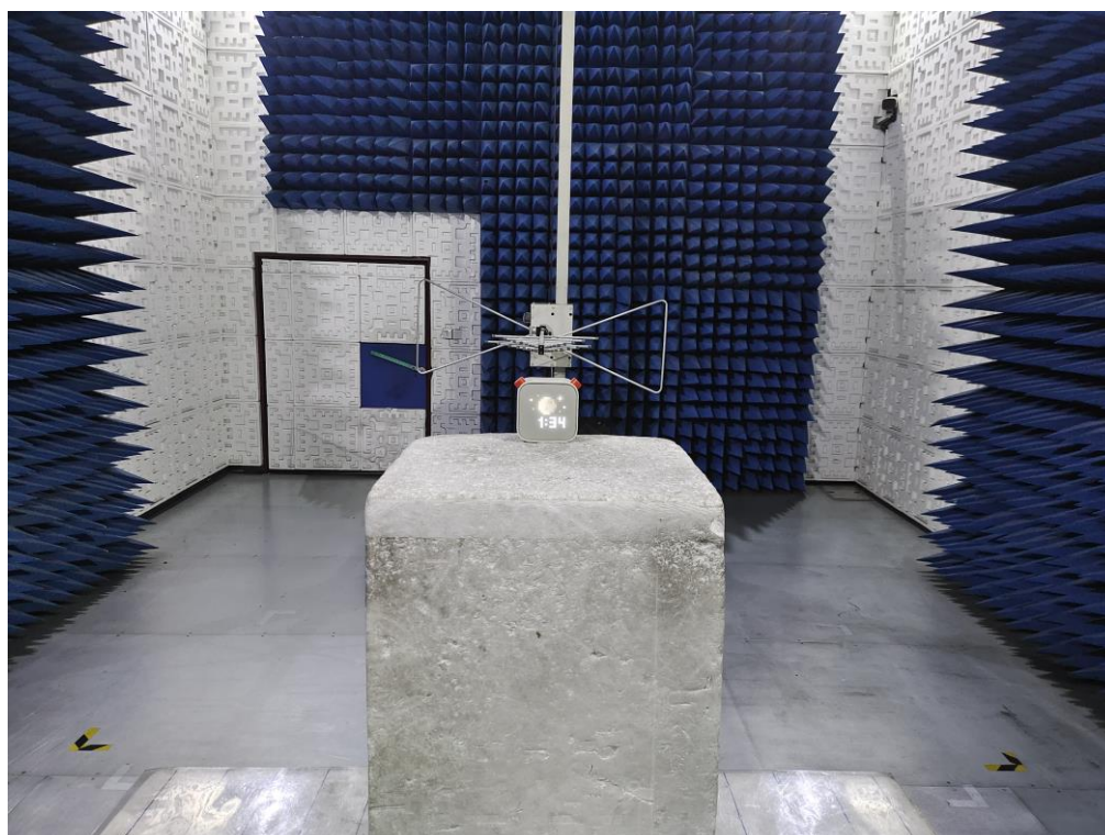
RADIATED EMISSION TEST SETUP ABOVE 1GHz
