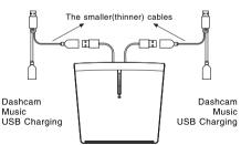
Please connect the wireless charger to the power-only cables (the smaller cables) of the USB splitters, not the power+data cables.
