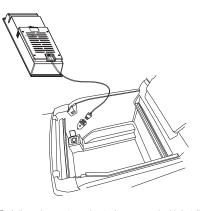
3.Push the car's own storage box to the passenger's side,install the Wireless Charger by aligning the front and rear grooves of the armrest box, slightly move and adjust it to fit with all parts of the
