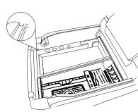
4. Turn on the switch of the Wireless Charger, and then place the phone compatible with QI standard on it to be charged. You can also pass the charging cable through the small hole in the
