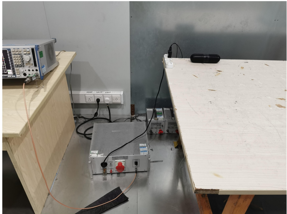
Conducted Emission Test Setup
