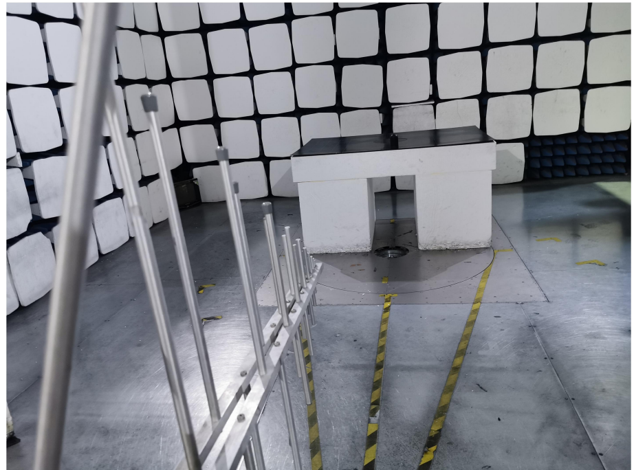
Radiation Emission Test Setup (30MHz to 1GHz)
