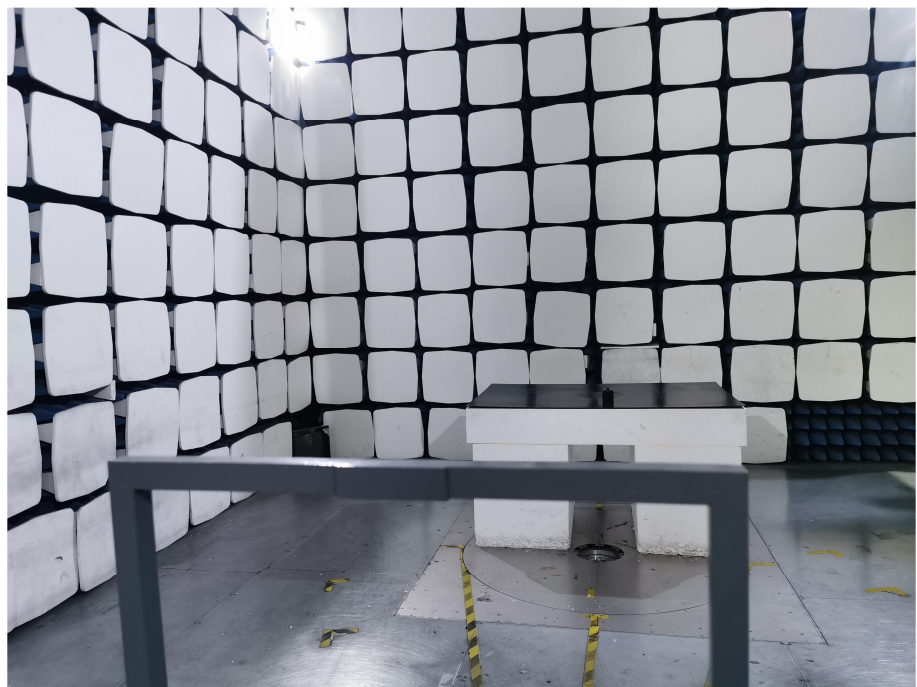
Radiation Emission Test Setup (Below 30MHz)
