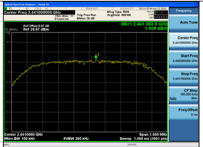
\pi/4 -DQPSK on Channel 39
