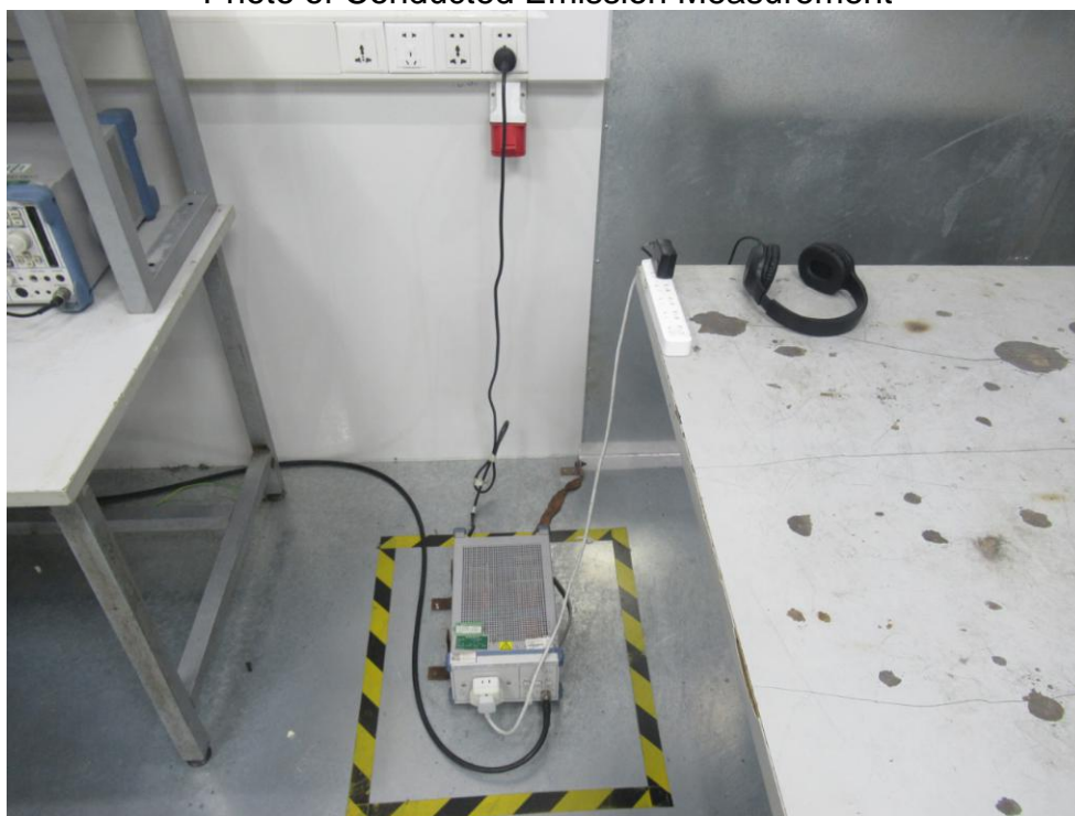
FCC ID: 2AS50-EBPD055 Photo of Conducted Emission Measurement
