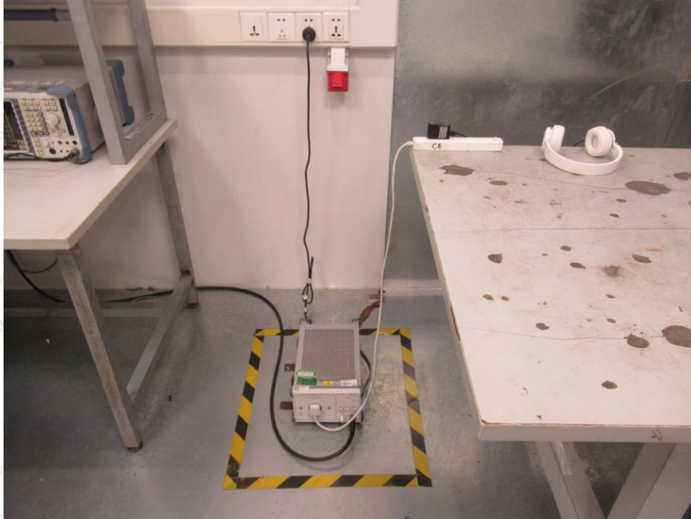
Photo of Conducted Emission Measurement
