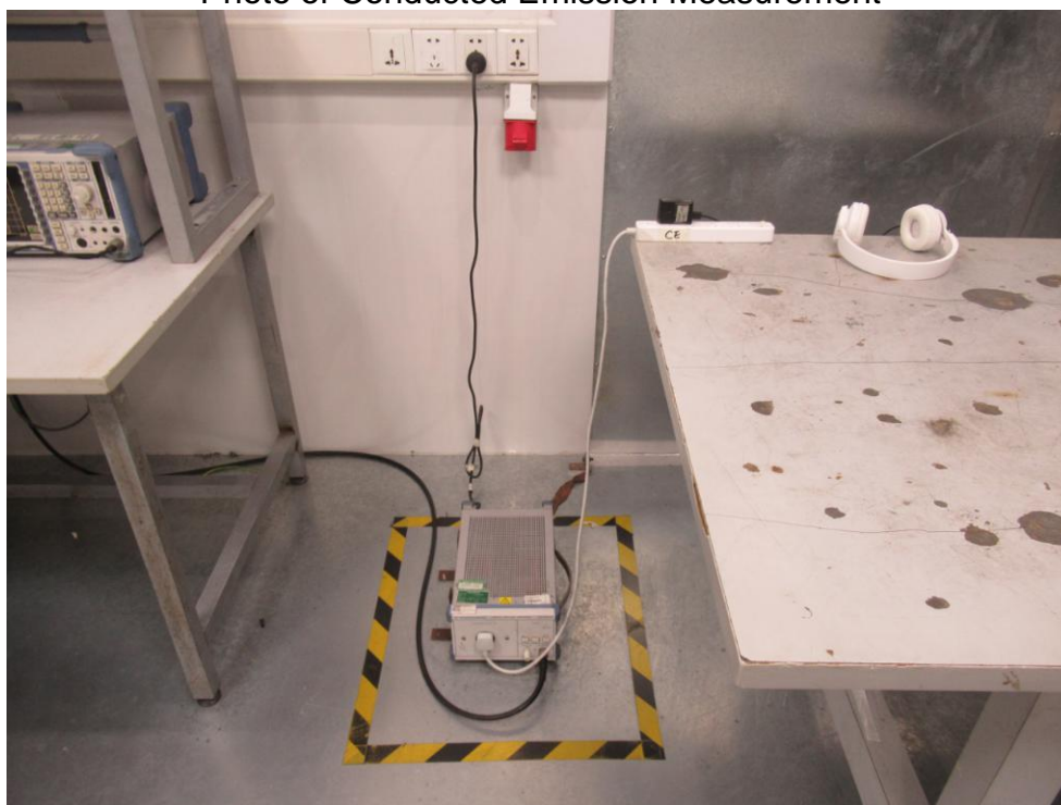
FCC ID: 2AS50-EBPD011 Photo of Conducted Emission Measurement
