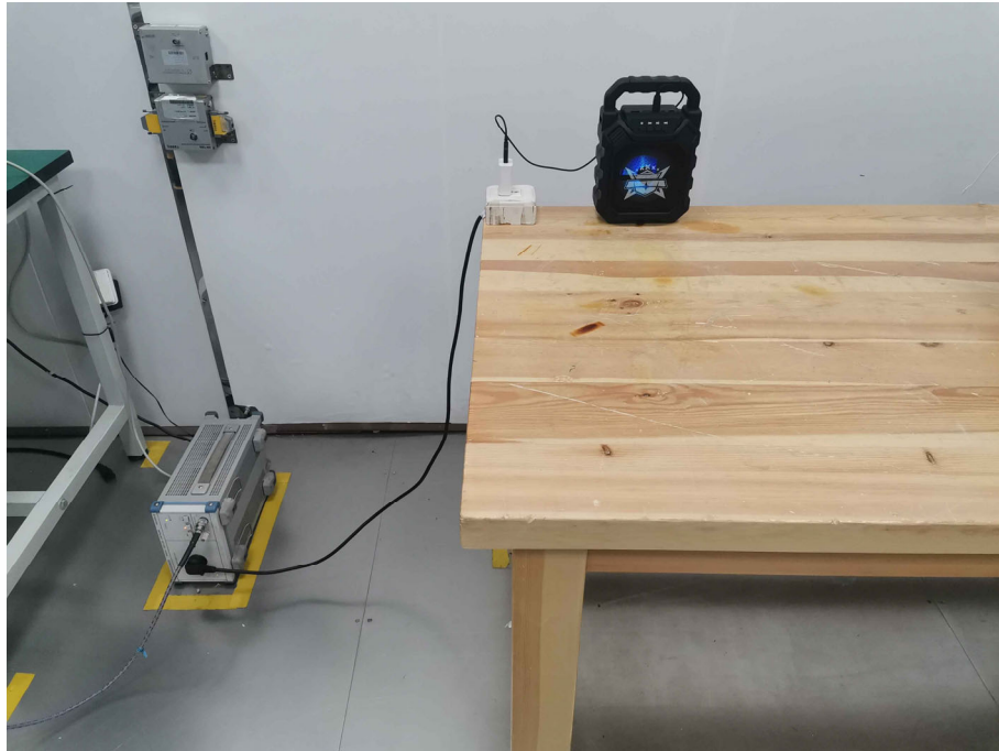
Conducted Emissions Test Setup
