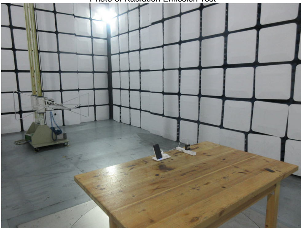
Photo of Radiation Emission Test
