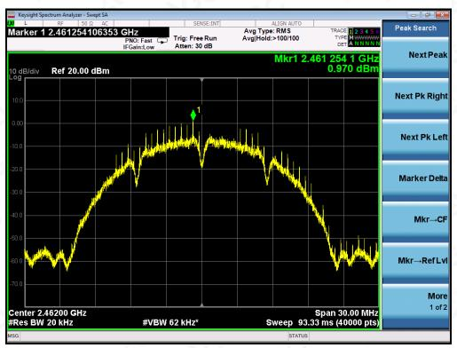
802.11g TEST RESULT TEST PLOT OF SPECTRAL DENSITY FOR LOW CHANNEL
