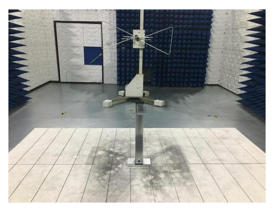
FCC RADIATED EMISSION TEST SETUP ABOVE 1GHZ
