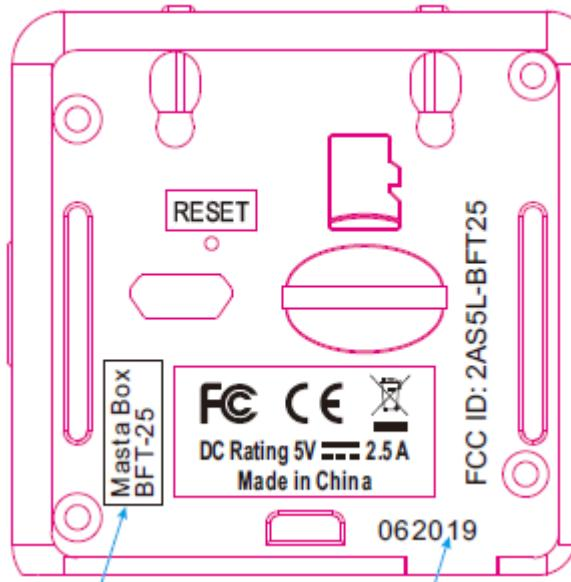
Specifications: Text is black in color and justified. Labels are printed in indelible ink on permanent adhesive silk-screened onto the EUT or shall be affixed at a conspicuous location on the EUT.
