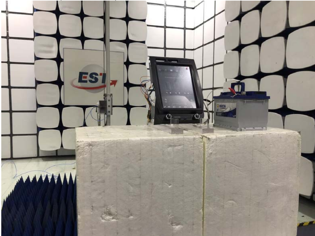
Radiated Test (Above 1GHz)
