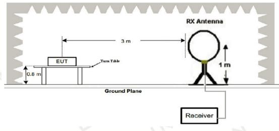
2. Radiated Emission Test-Up Frequency 30MHz~1GHz
