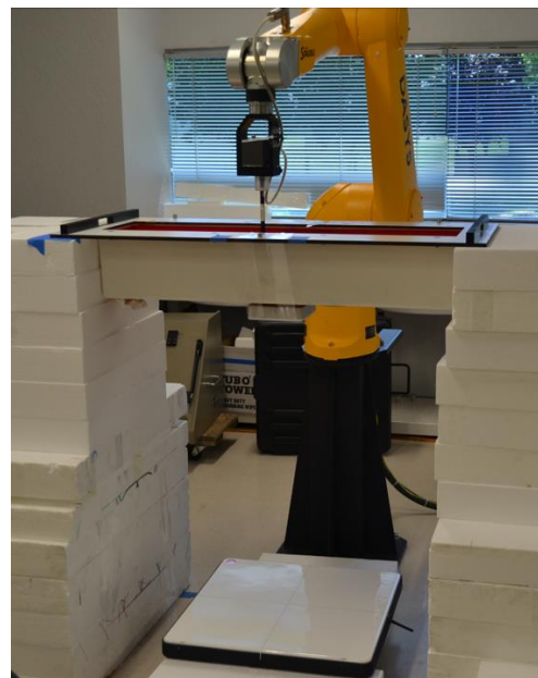
Figure 16 - SAR measurement test setup
