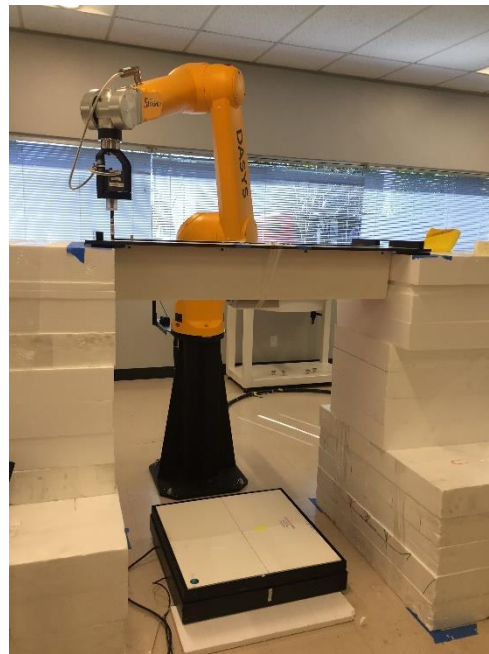
Figure 94 - SAR measurement test setup
