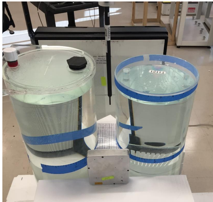
Figure 74 - photo of two phantom test configuration
