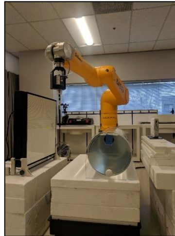
Figure 57 - Test setup - single phantom, transverse orientation (75 cm)
