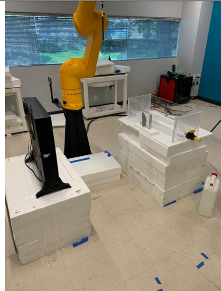
Figure 88: Half-cylinder phantom behind WPT client
