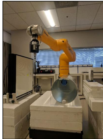
Figure 45 - Test setup - single phantom transverse plane
