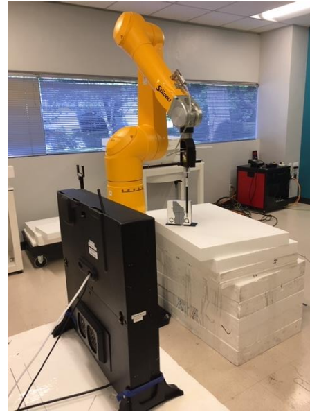
Figure 23 - Power source angle: 45° Client angle: 0° scan closest to WPT Source - Horizontal plane
