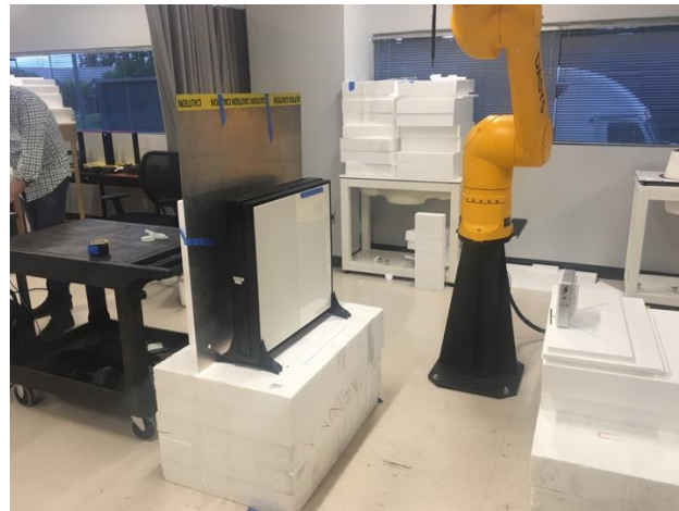
Figure 37: Test setup - metal plate behind WPT Source
