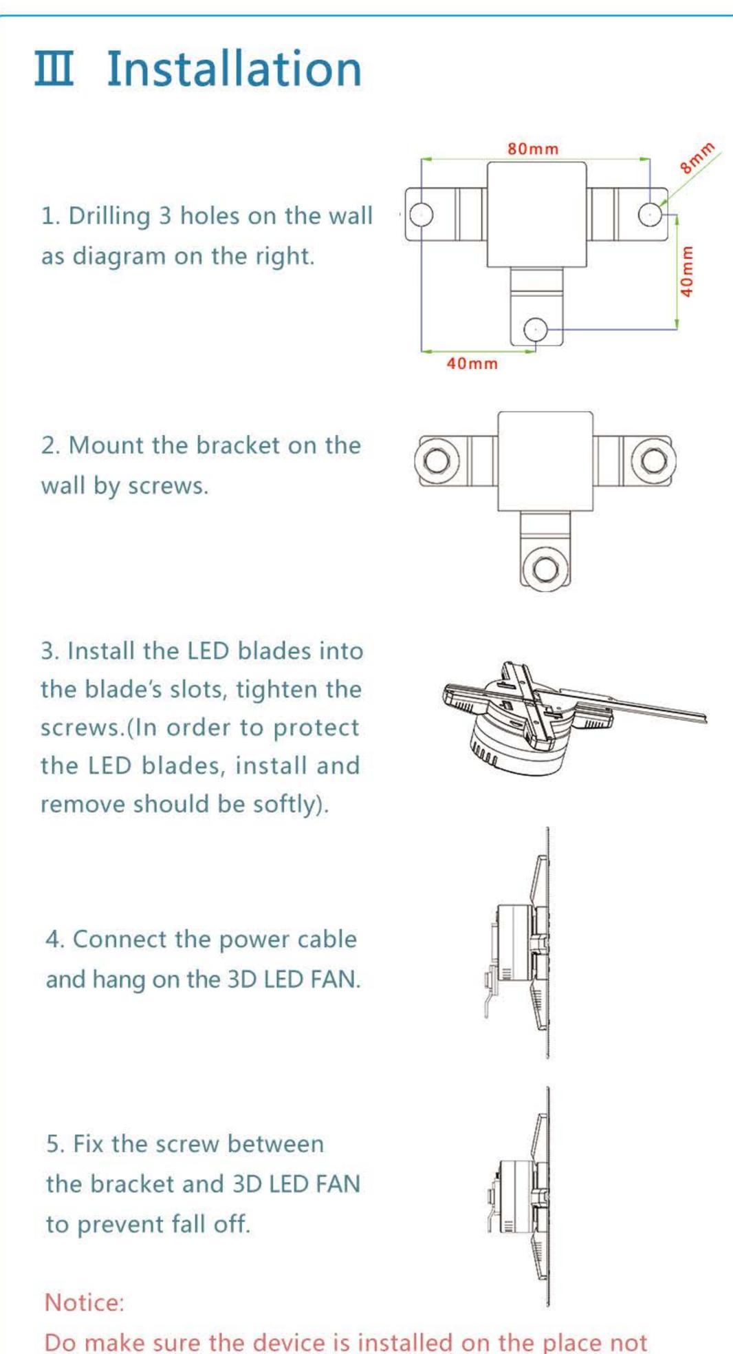
Do make sure the device is installed on the place not touchable, or it must need a protection cover to keep safety.
