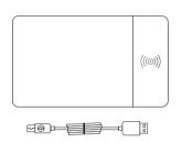
2. Insert the small end of the USB charging cable into the Micro USB port of the wireless charging mousepad. The LEDs indicate connectivity.
