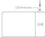
3. Place your Qi-standard device on the wireless charging mousepad area to start wireless charging. LED lights will start pulsing, below, or use an available USB port. indicating the device is charging.
