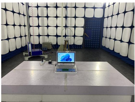
3. Radiated emission (9KHz-30MHz)
