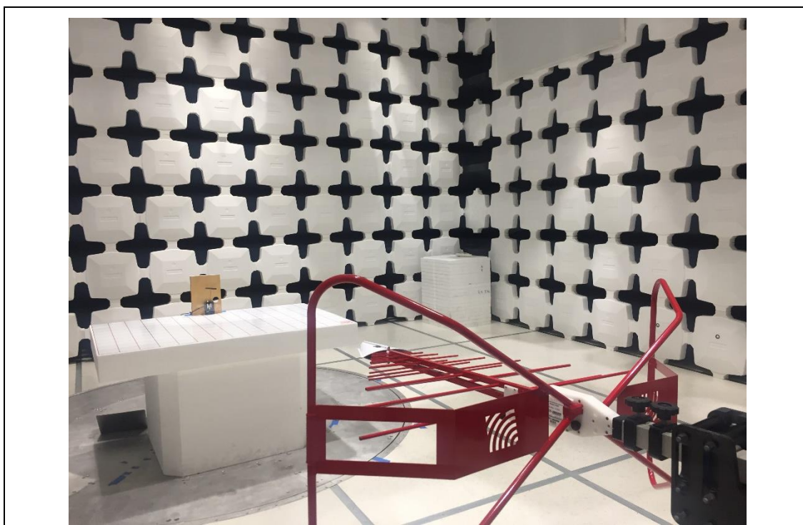
Radiated Emissions Below 1GHz setup – Front
