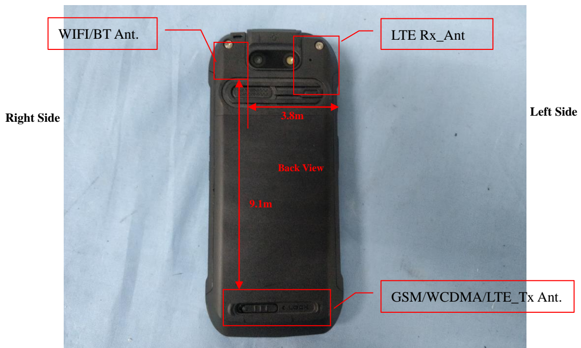
Block Diagram for EUT Antenna Position
