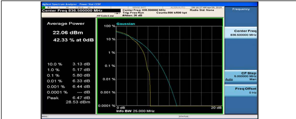
Channel Bandwidth: 10 MHz_MCH_16QAM_25RB#0
