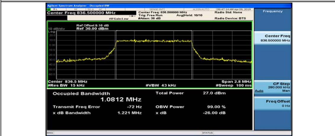
(Channel Bandwidth: 1.4 MHz)_MCH_16QAM_6RB#0
