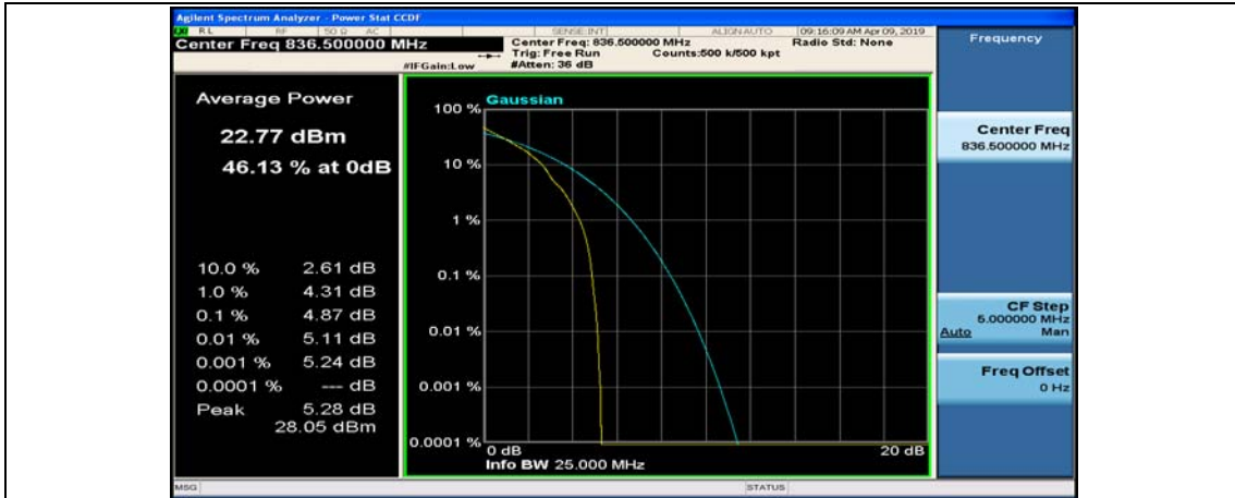
Channel Bandwidth: 10 MHz_MCH_QPSK_25RB#0
