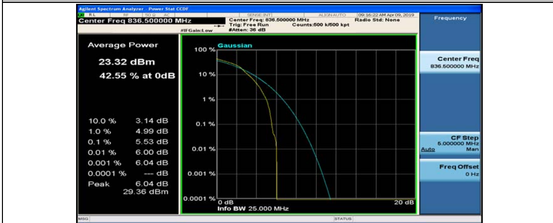
Channel Bandwidth: 10 MHz_MCH_16QAM_1RB#49
