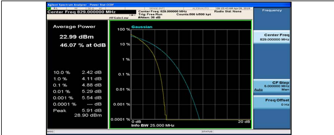
Channel Bandwidth: 10 MHz_MCH_QPSK_1RB#0
