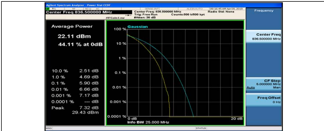
Channel Bandwidth: 10 MHz_MCH_QPSK_50RB#0
