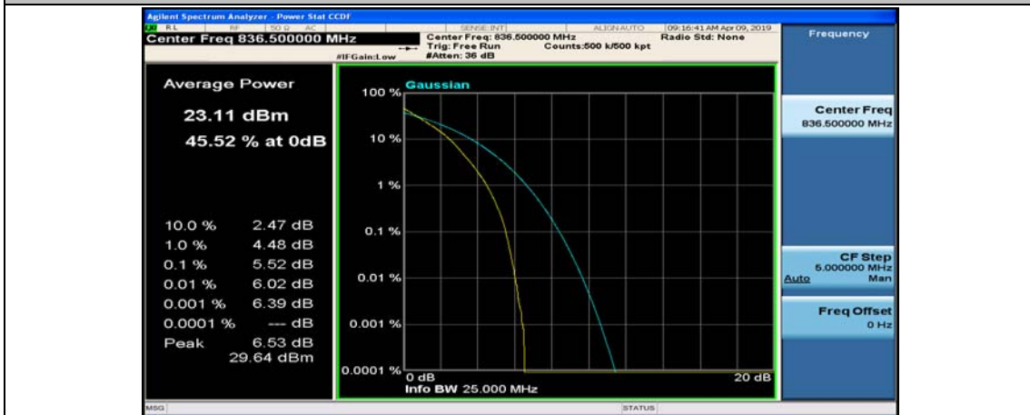
Channel Bandwidth: 10 MHz_MCH_QPSK_25RB#25
