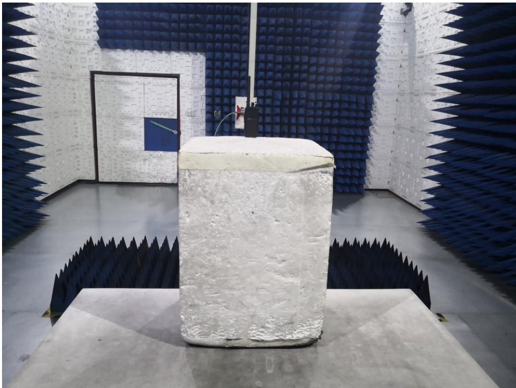
RADIATED EMISSION TEST SETUP ABOVE 1GHz
