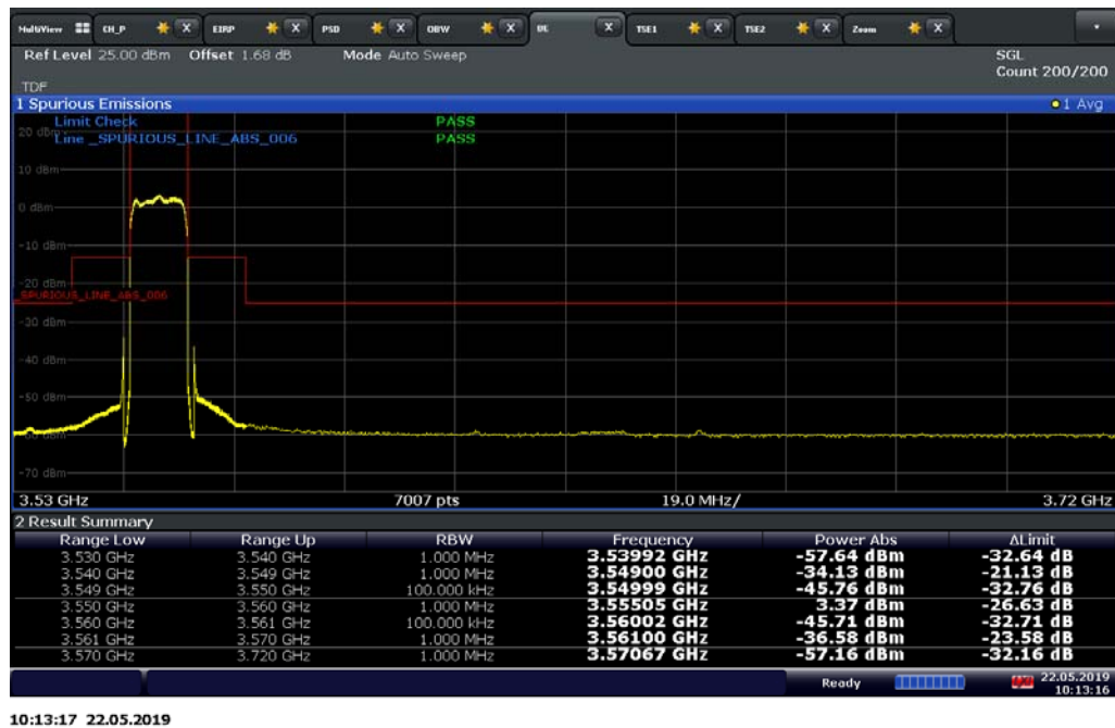
LTE Band 48 / 10 MHz / 16QAM
