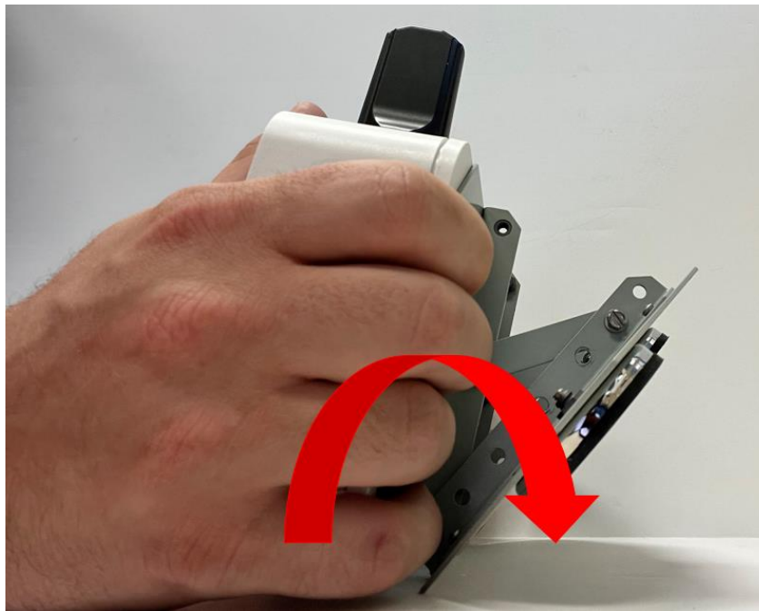
Figure 15: Rolling the magnet mount onto the magnetic surface
