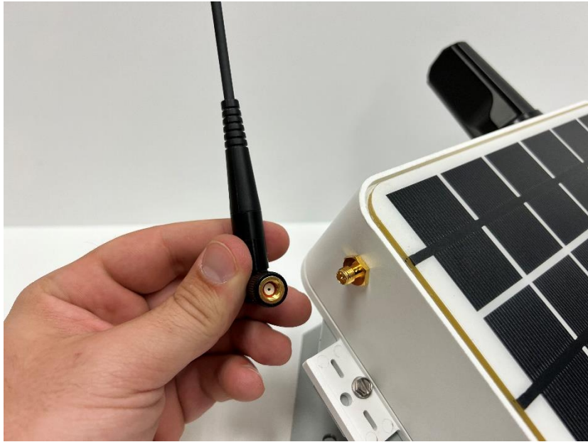
Figure 10: LoRa antenna and SMA connector
