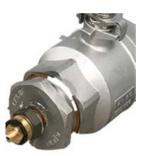
2. The DGA LT1 is designed for a 1" drain valve however bushings are optionally provided with the DGA-LT1 to install into a 2" drain valve. The bushings should be installed with pipe dope or Teflon tape to ensure a seal
