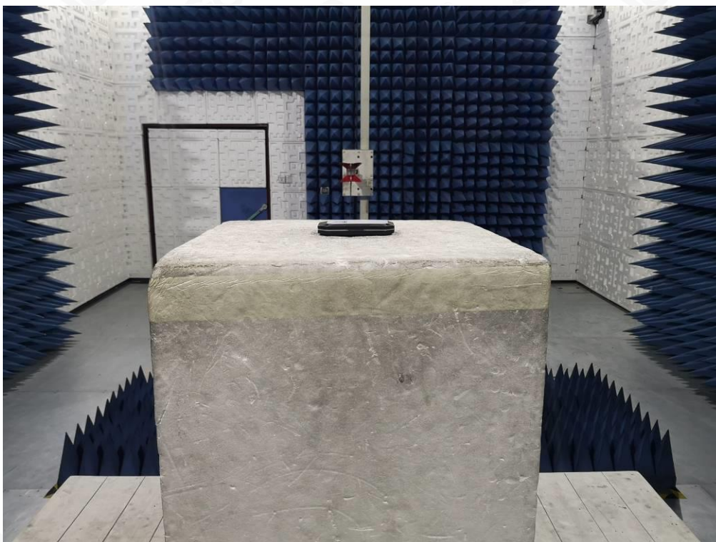
FCC RADIATED EMISSION TEST SETUP ABOVE 1GHZ
