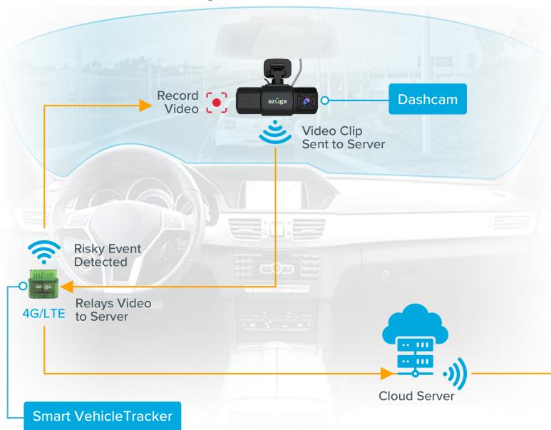
Azuga SmartCam<sup>™</sup> is a smart device connected to Azuga SmartVehicle device integrated with our Azuga Fleet Mobile & Web App that records videos only when it is necessary so you are alerted only when necessary instead of watching a video of the entire trip.
