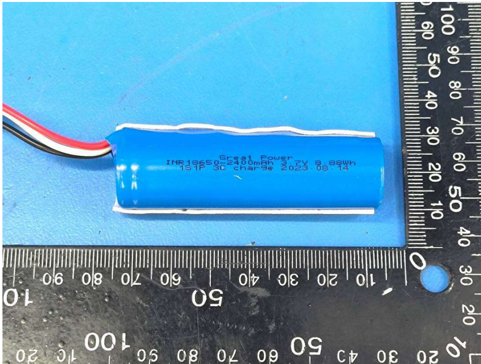
Internal lithium battery view
