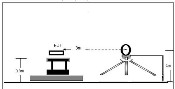
(B) Radiated Emission Test-Up Frequency 30MHz~1GHz
